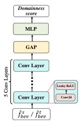
Figure 4. Detailed structure of domain discriminator.  $\hat{f}^s_{bev}$  and  $\hat{f}^t_{bev}$  denote enhanced foreground features from source domain and target domain.
